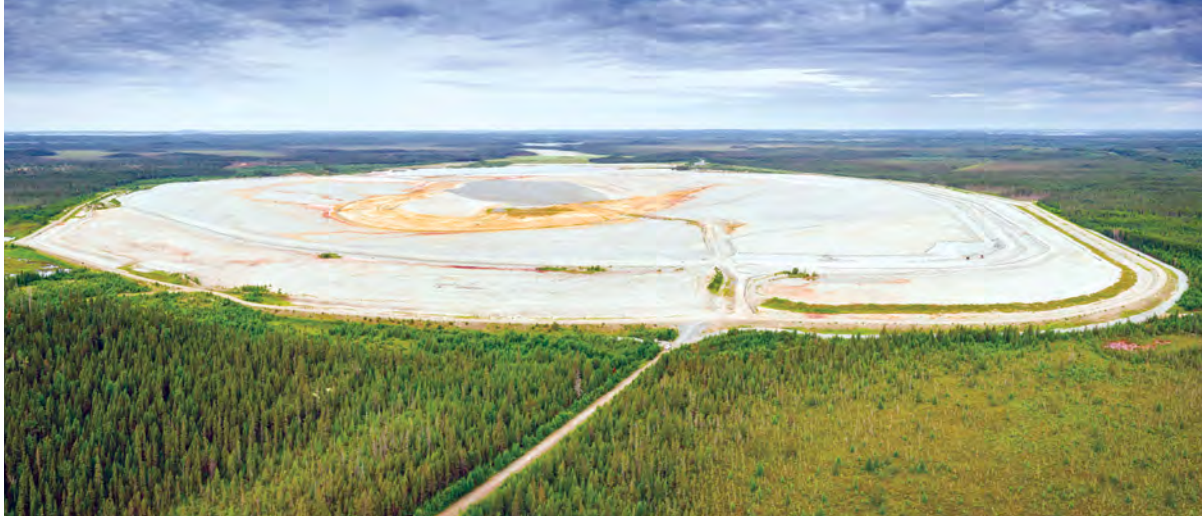
Agnico Eagle and the Government of Quebec came up with an innovative solution to an environmental problem being caused by the orphaned Manitou acid-generating tailings facility by using sulphide-free and cyanide-free tailings produced by the Goldex mine to cover the tailings.
